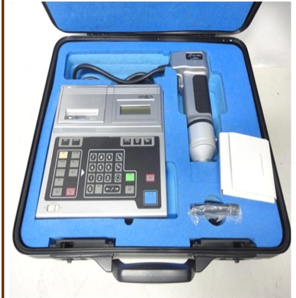
*Colorimeter( color-difference meter)
